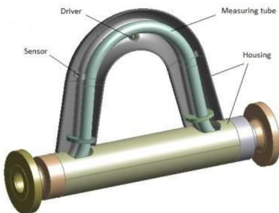
Figure 1: Inside view of a Coriolis mass flowmeter.
